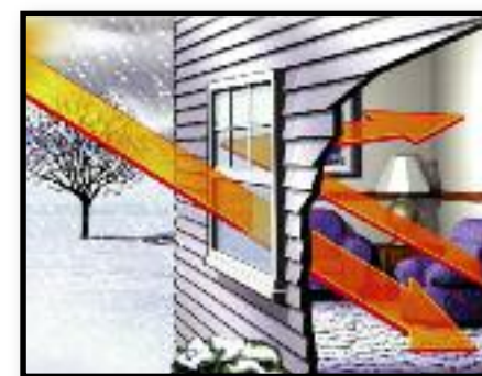
Low-E glass takes on a new responsibility in winter months. It lets warm solar rays into your home, while blocking the heat inside of your home from getting out.
