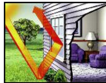
Low-E glass filters long-wave radiation from the sun. This reduces solar heat gain from the summer sun, helping to keep your home cooler.
